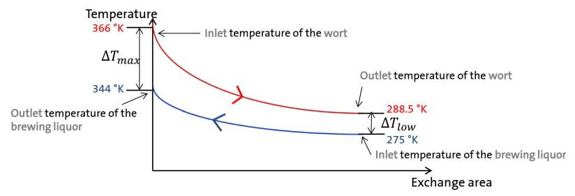
For that purpose, the average logarithmic temperature  $\Delta T_{log}$  is used for calculations:
