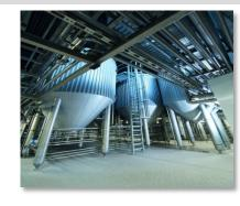
No cooling energy required! During respiration and fermentation, yeast releases heat that helps to reach the primary fermentation temperature within a day.
