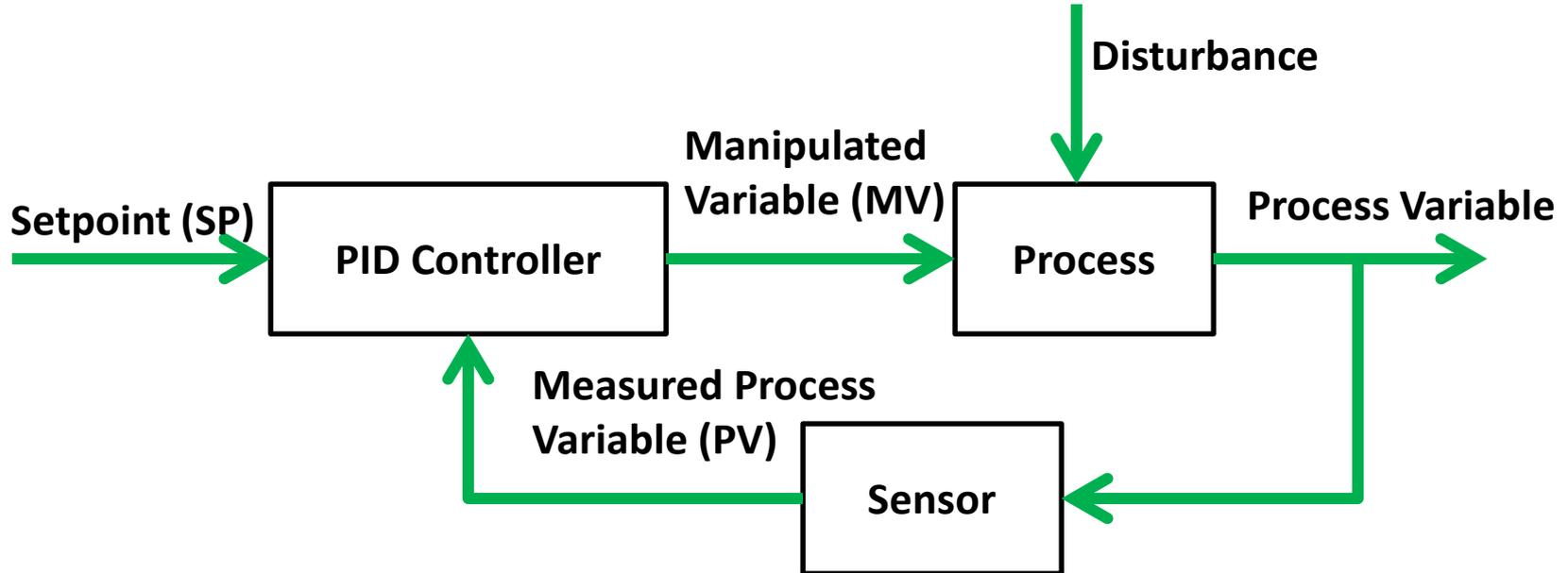
Classic block diagram of a PID Loop
