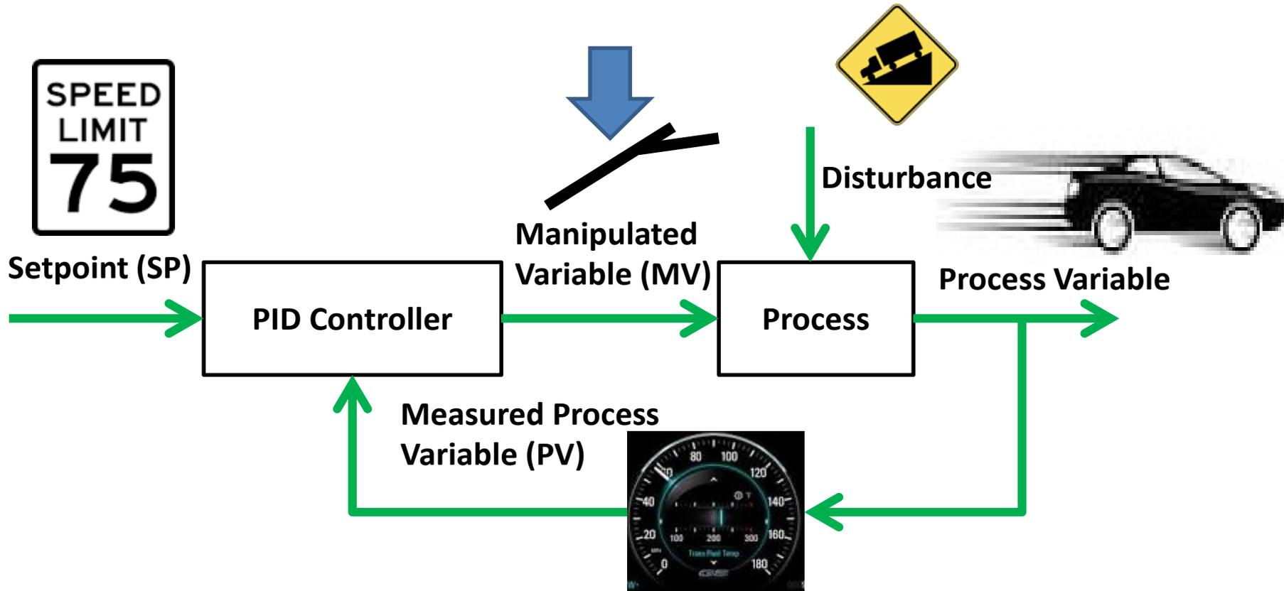
Block diagram of a Cruise Control PID Loop
