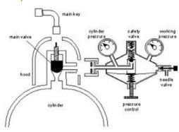
Cylinder valves are made of brass and can easily break off. This could cause the high pressure within the cylinder to release violently, causing it to become a dangerous torpedo capable of going through walls. Visual inspect your valves and regulator frequently. See OSHA 1910.101 for more details.
